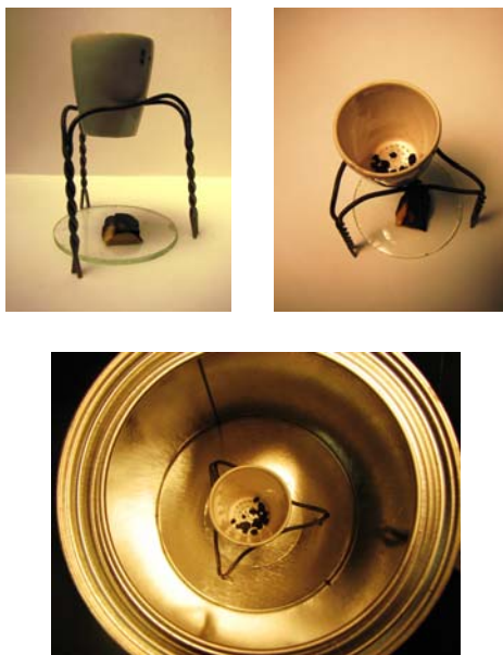
Figure 2. Crucible positioned over fire debris sample in wire triangle. Side view, top view and placement in paint can.
